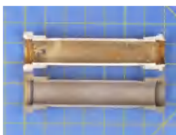
the sample after sectioning longitudinally and mechanical cleaning of one half.
