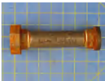
The Carbon Steel Spool Piece As-Received. The sample was found to be in good condition
