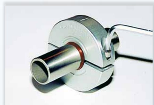
Step 4. Retighten both halves of the ring. Do not over tighten.
